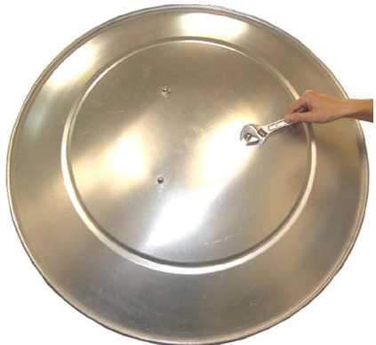
Figure 12 - Attaching Dome to Burner Assembly
